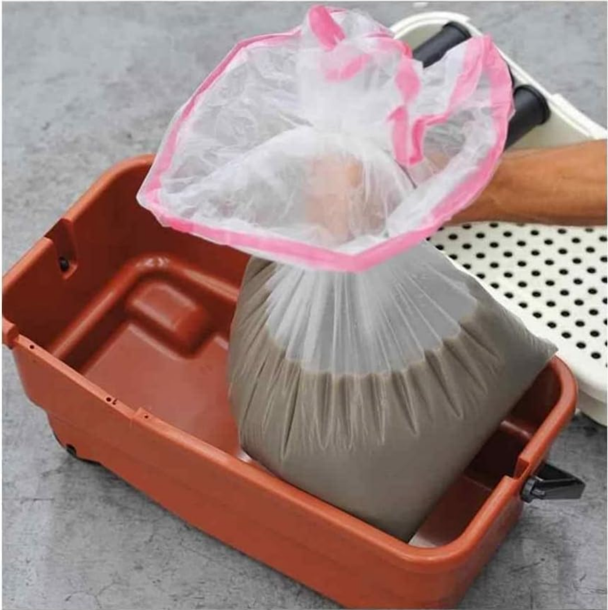
Figure 3: A disposable liner bag filled with dirty water and grout slurry, ready for removal and disposal.
