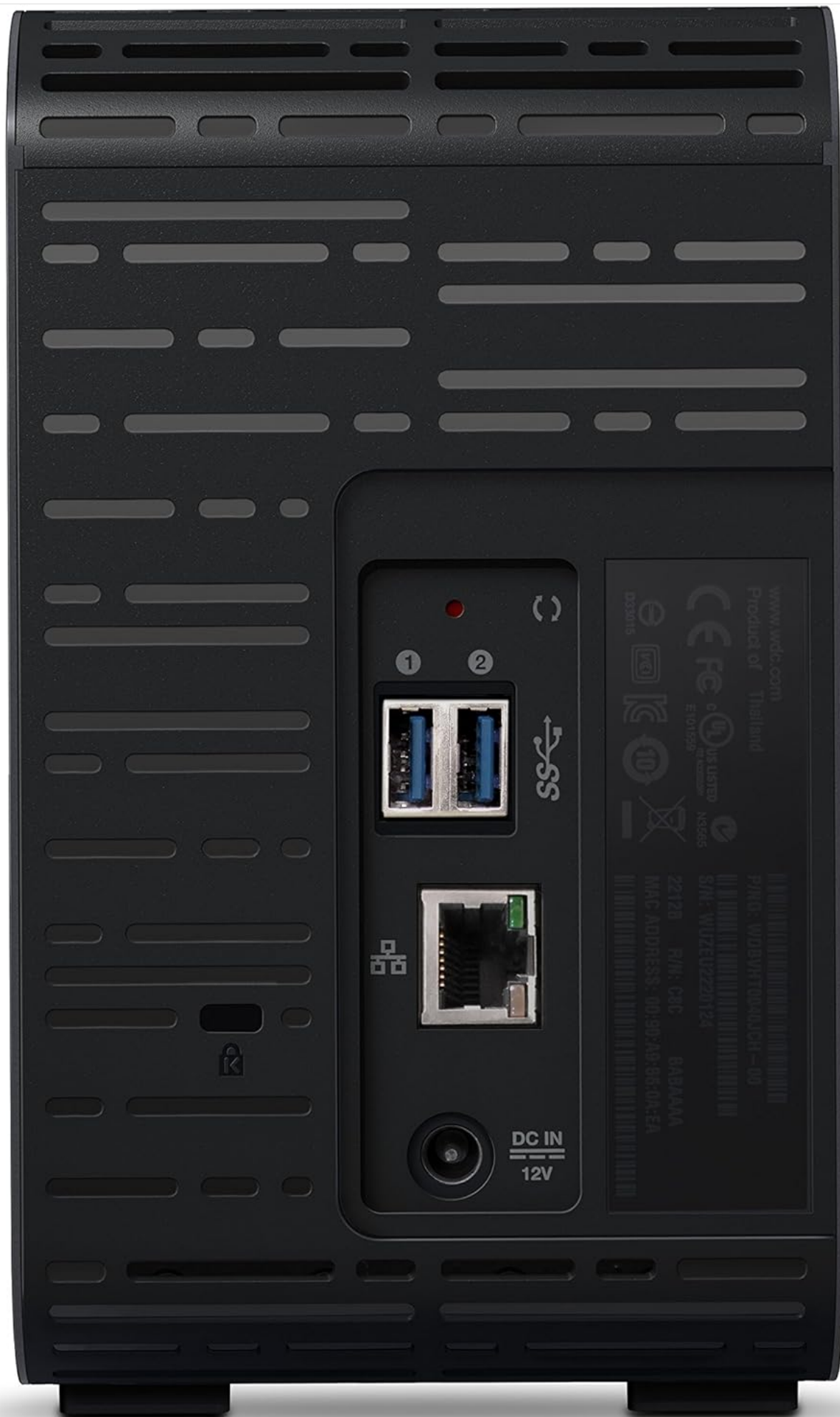
Image: The rear panel of the My Cloud EX2 Ultra, highlighting the Ethernet port, USB 3.0 ports, and power input for connectivity.
