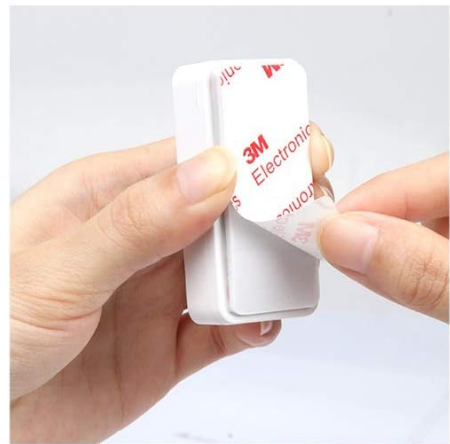
Step2: Install the transmitter(stick with provided double-sided sticker)
