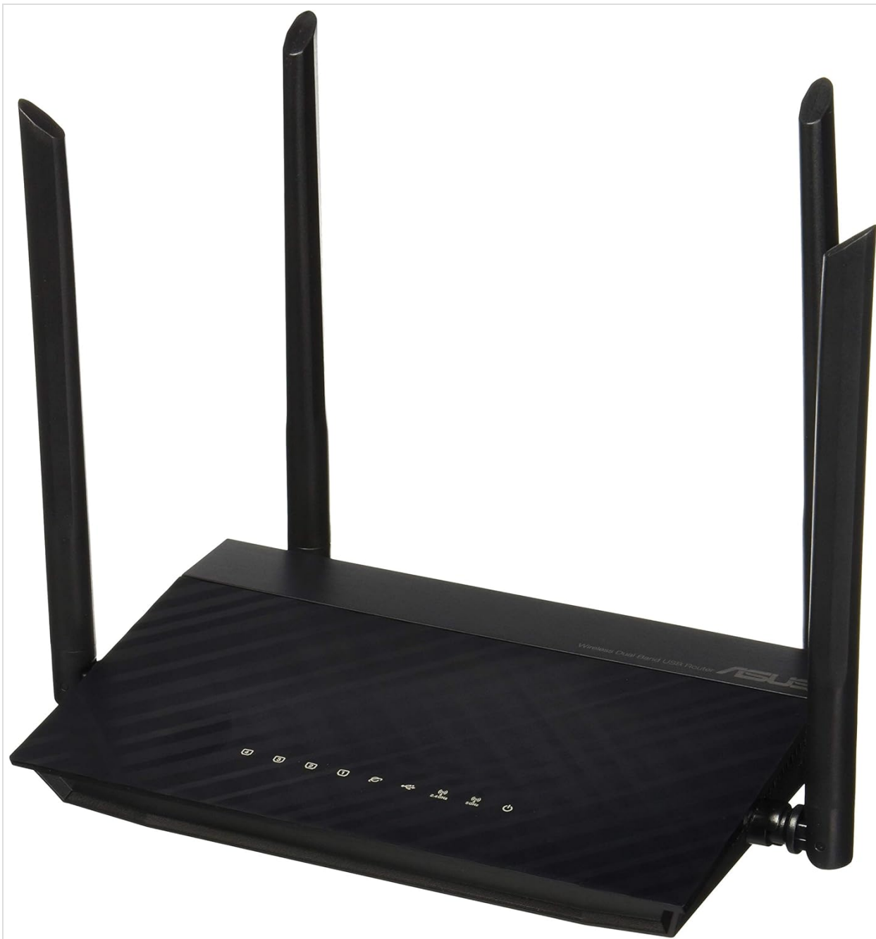
Figure 2.1: Front view of the ASUS RT-AC1200 Wireless AC1200 Dual-Band Router, showing its four external antennas and indicator lights.
