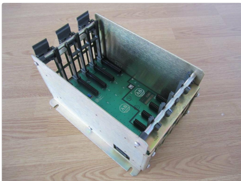
Figure 2.1: Angled view of the Allen Bradley 1771-A1B 4-Slot I/O Chassis, showing the module slots and backplane.
