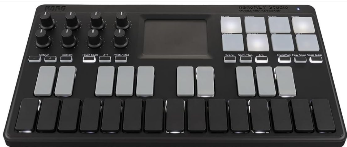
Figure 2.2: A top-down view of the KORG nanoKEY Studio, highlighting its keys, pads, knobs, and X-Y touchpad for a clear understanding of its interface.
