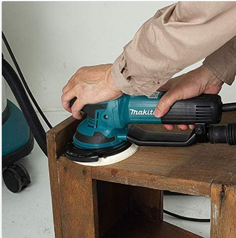
Figure 5.2: The Makita BO6050J Eccentric Rotary Sander being used by a person to sand a wooden cabinet. The sander is connected to a dust extraction system, visible in the background.
