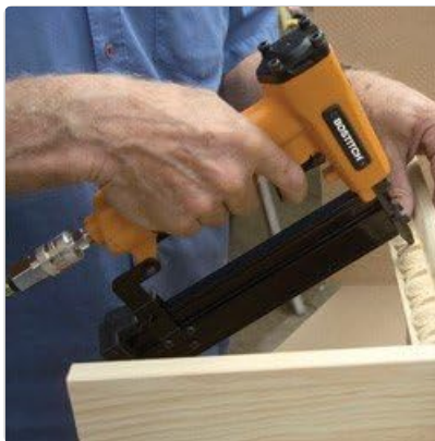
Figure 2: The Stanley Bostitch MB2140-E Pin Stapler being used to fasten wood. This image demonstrates the proper grip and positioning of the tool during operation.
