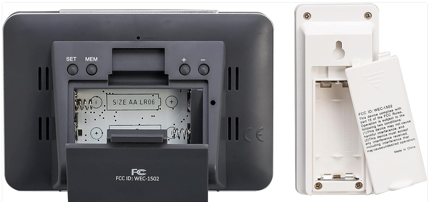
Image: Rear view of the main unit and remote sensor, showing their respective battery compartments open for battery insertion.
