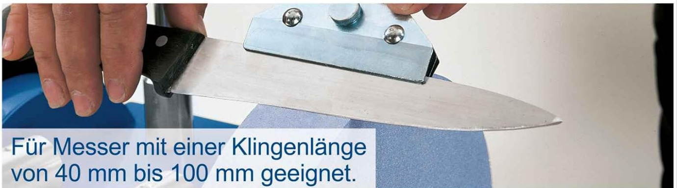
Figure 5.5: Optional jigs for sharpening curved blades, tubes, hollow irons, and knives with blade lengths from 40 mm to 100 mm.
