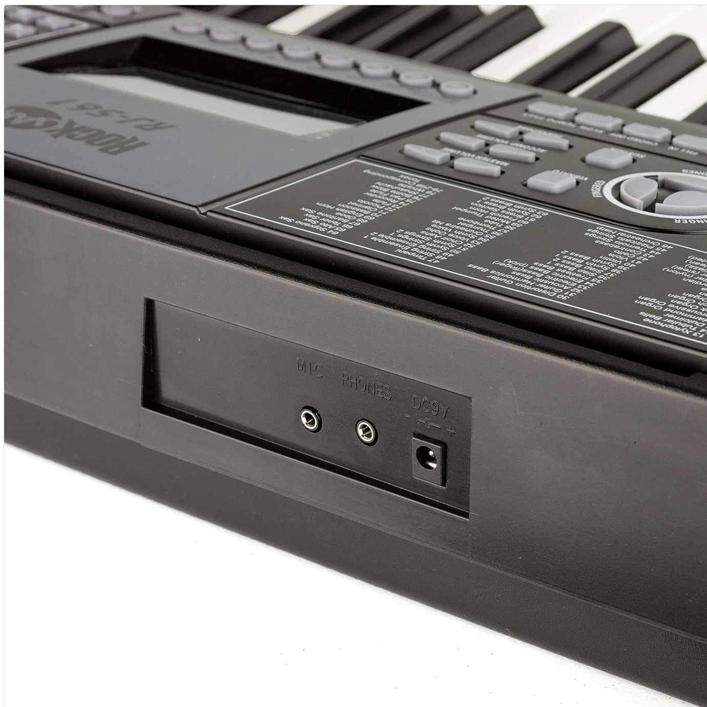
Figure 3.3: Rear panel connections for power and headphones.
