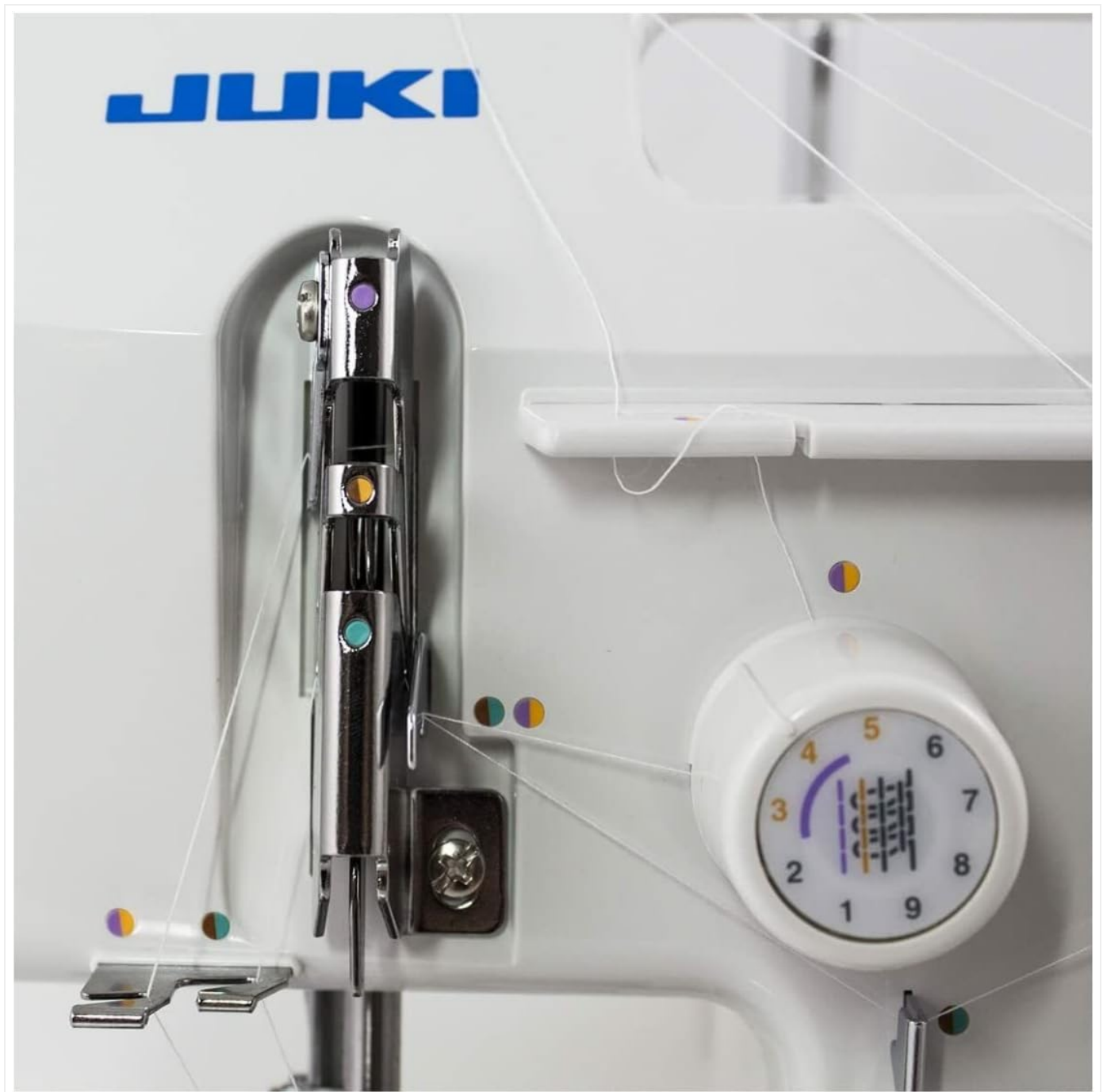
Figure 5: Needle area threading. This image provides a detailed view of the needle bar, presser foot, and the final threading points for the needles and loops.
