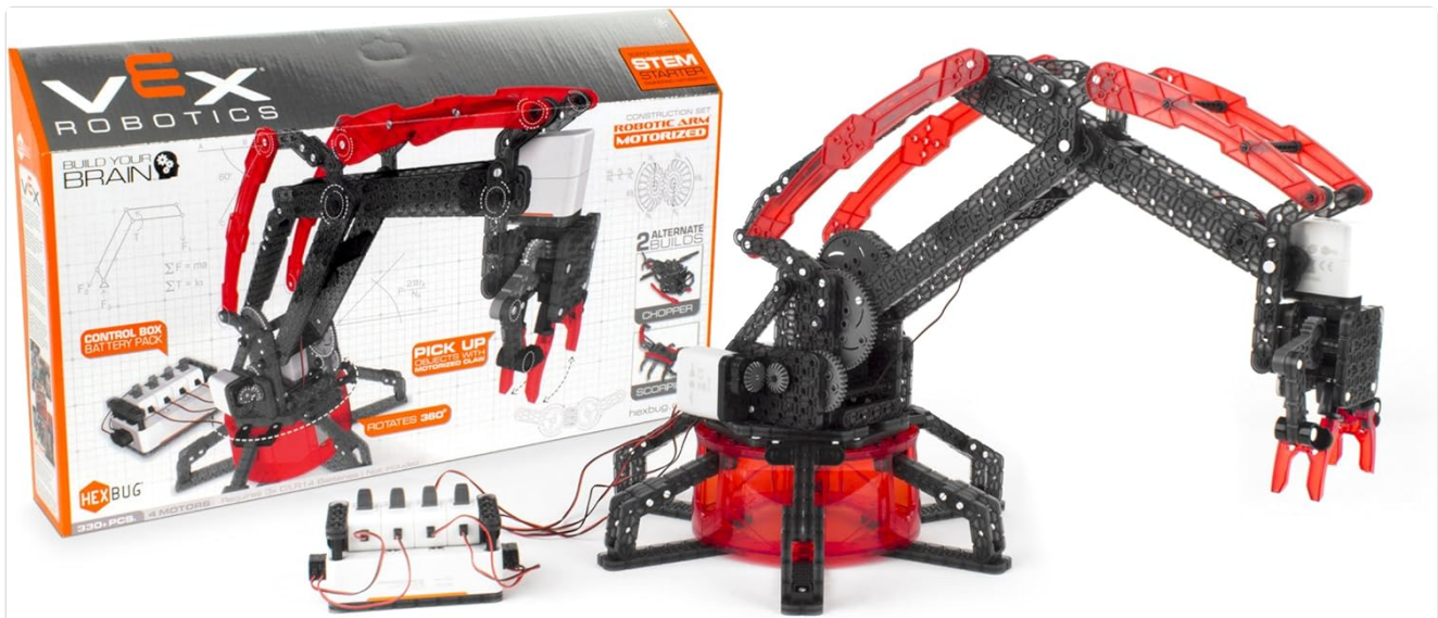
Image 4.1: The VEX Robotics kit, showing the packaging and the assembled robotic arm, ready for operation.
