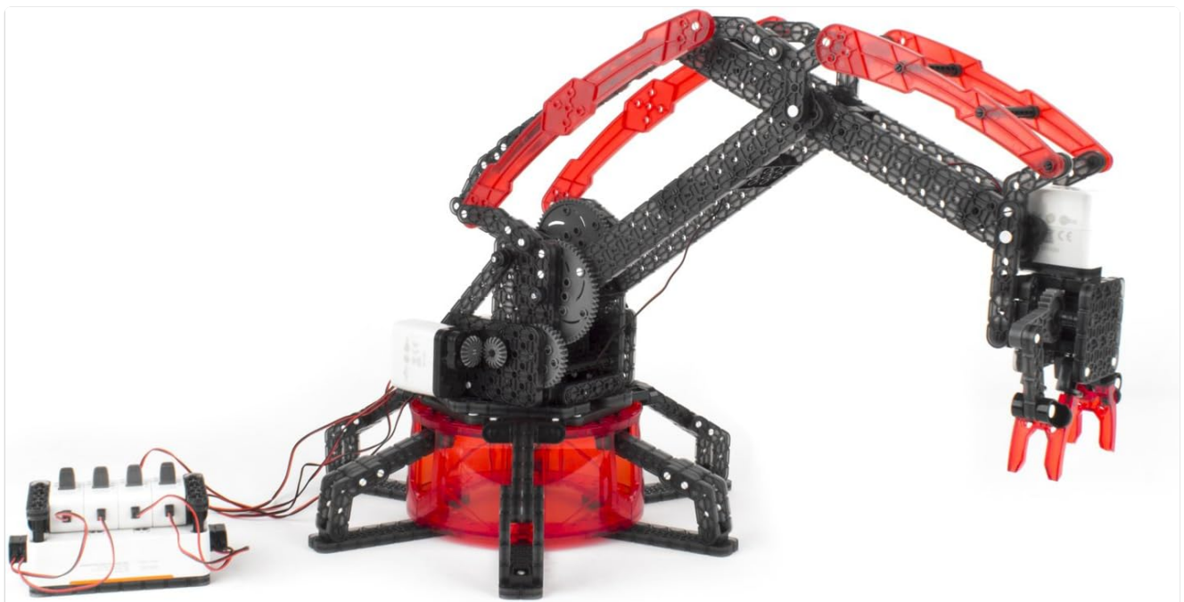
Image 1.1: The fully assembled HEXBUG VEX Robotics Motorized Robotic Arm, showcasing its articulated structure and control box.
