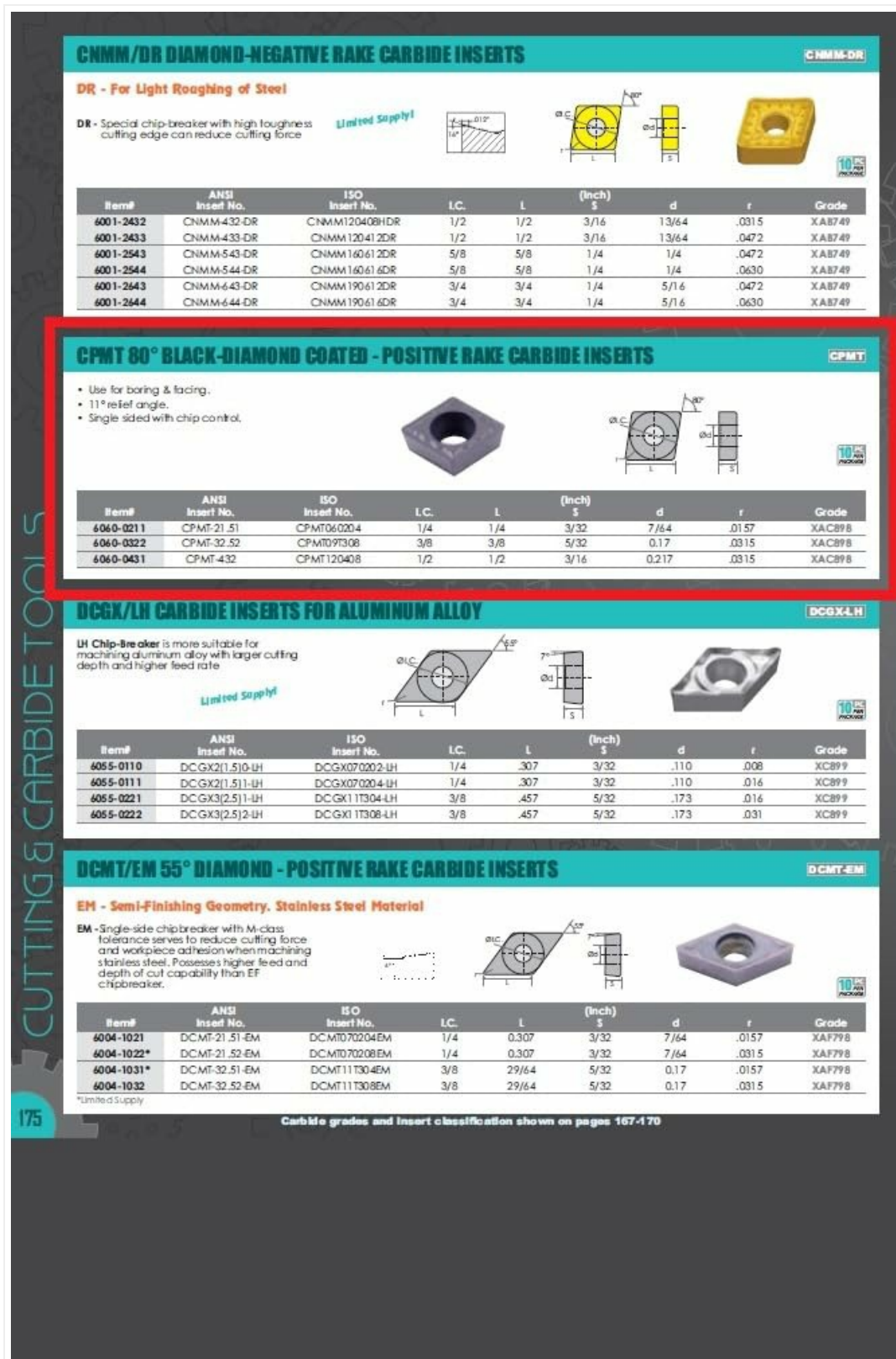
Figure 2.3: A section from a carbide insert selection chart, specifically highlighting the CPMT 80° Black-Diamond Coated Positive Rake Carbide Inserts. This chart helps in identifying the specific insert type and its general characteristics.
