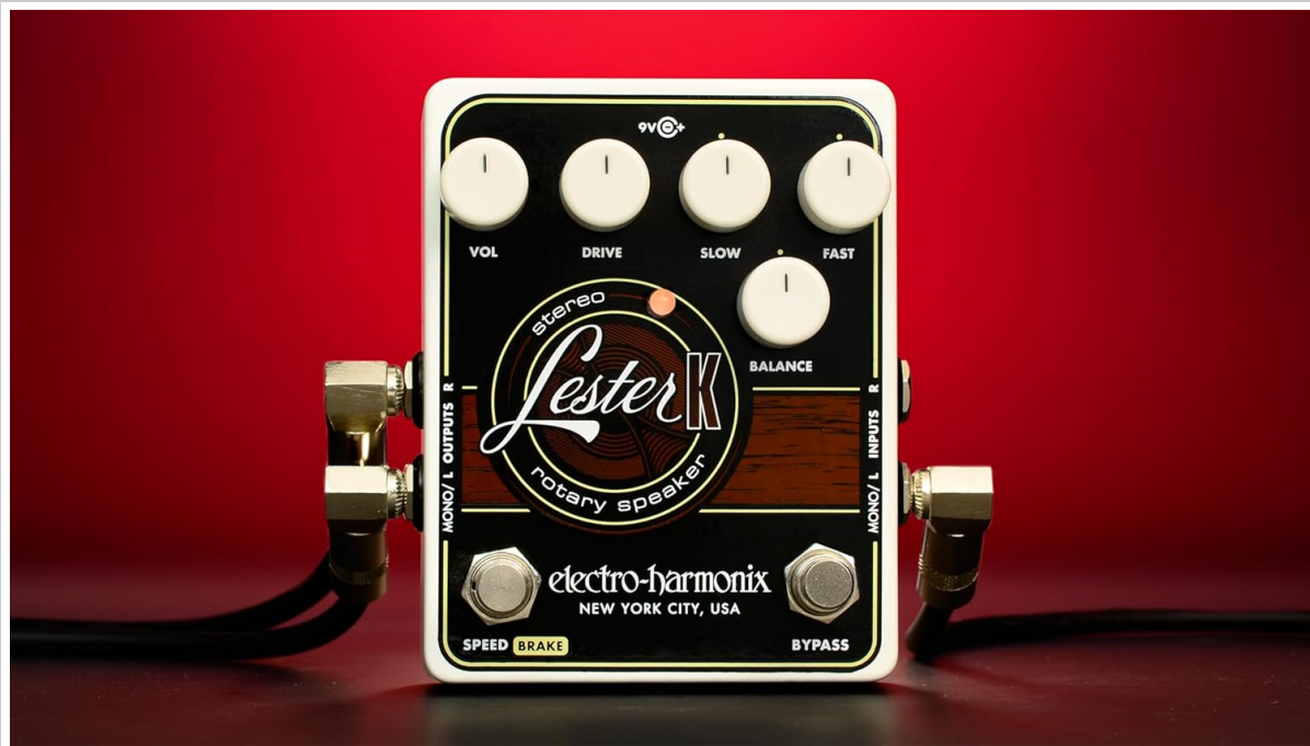
Image: A clear view of the Lester K's control layout, including the VOL, DRIVE, SLOW, FAST, and BALANCE knobs, and the SPEED/BRAKE and BYPASS footswitches.
