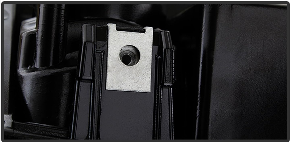
Image 4.3: Detail of a mounting bracket on the tail light assembly, indicating attachment points.
