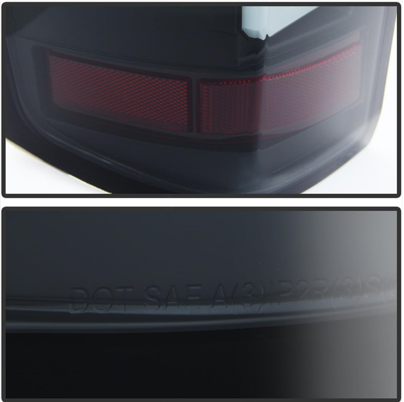
Figure 9.2: Detail of the tail light's lower section, including reflector and compliance markings.
