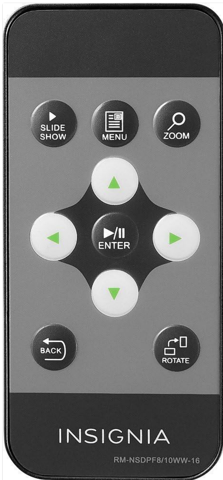
Image: The remote control for the digital photo frame, featuring dedicated buttons for slideshow, menu, zoom, directional navigation, enter, back, and image rotation functions.
