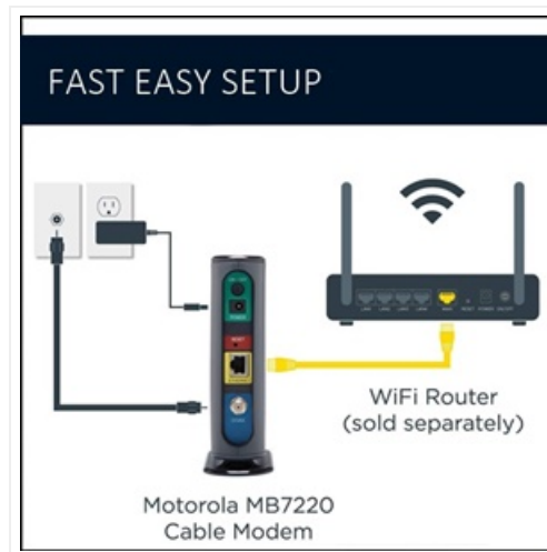
Image 3.2: Diagram illustrating the connection process for the Motorola MB7220 Cable Modem to a wall outlet, power, and a WiFi router.
