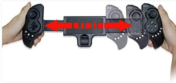
Figure 4.1: The telescopic mechanism of the iPega PG-9023, demonstrating how it expands to accommodate different device sizes.
