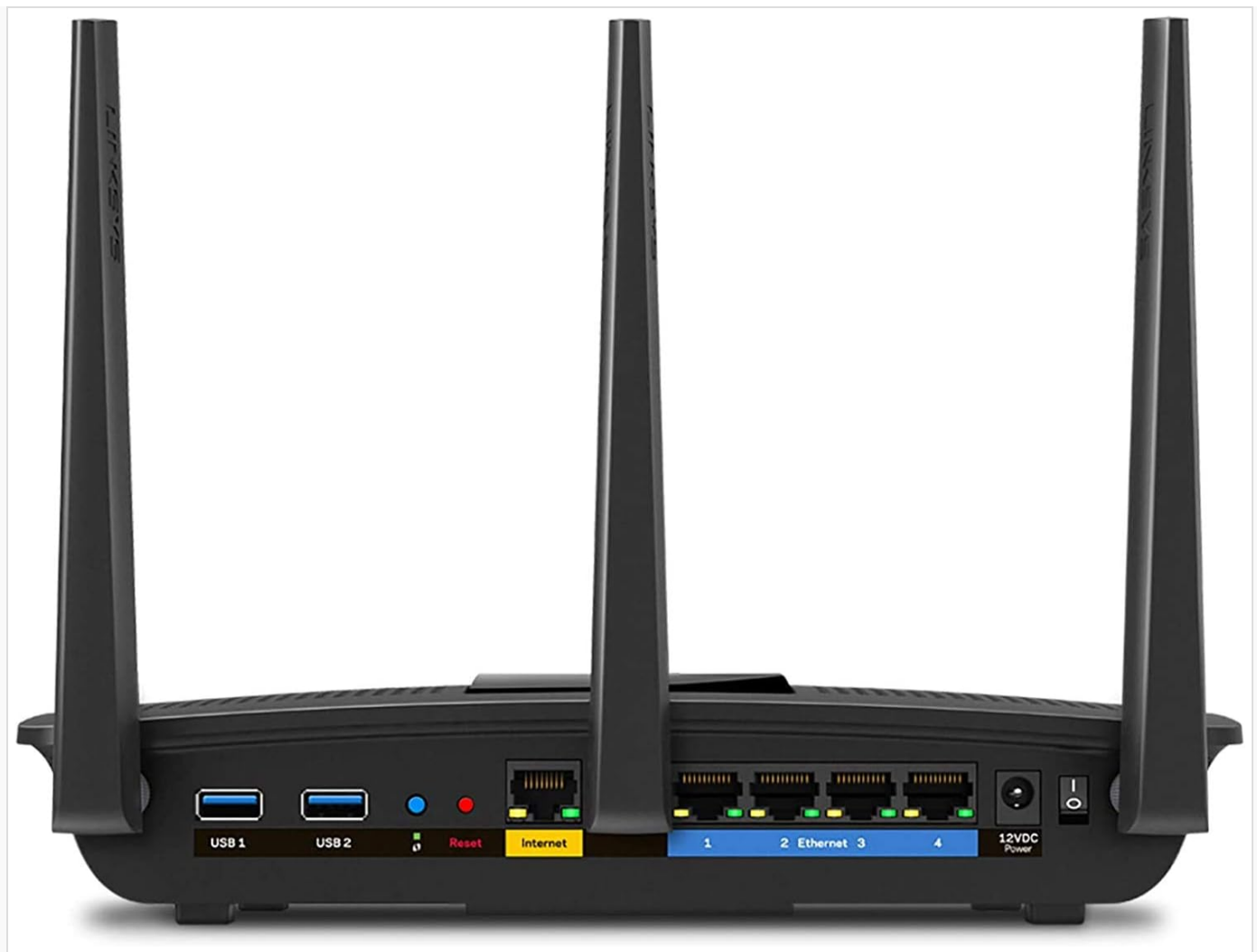
Figure 3.2: Rear view of the Linksys EA7500 router, detailing the USB 1, USB 2, Reset button, Internet (WAN) port, four Gigabit Ethernet (LAN) ports, 12V DC power input, and Power On/Off switch.
