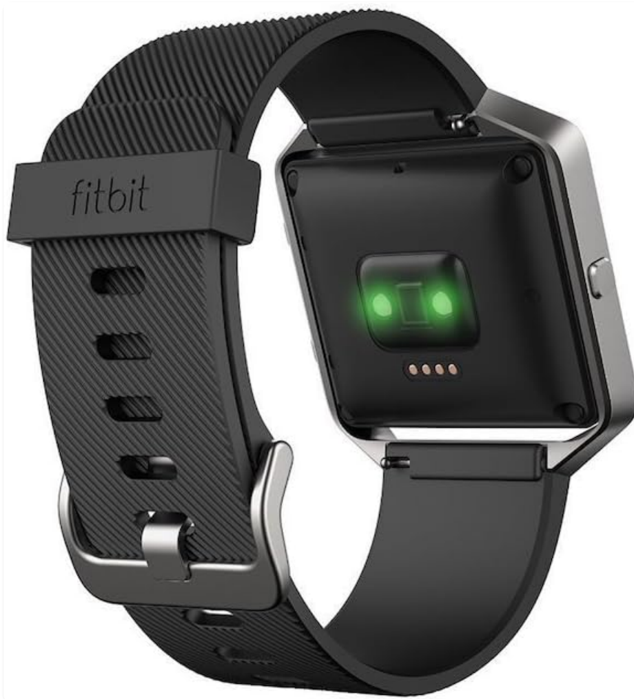
Figure 2: Rear view of the Fitbit Blaze, highlighting the PurePulse heart rate sensor.
