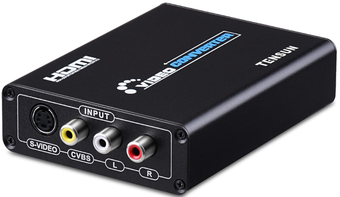
Image: Front view of the Tensun HDMI Converter, showing the S-Video, CVBS (yellow), and R/L audio (white, red) input ports.
