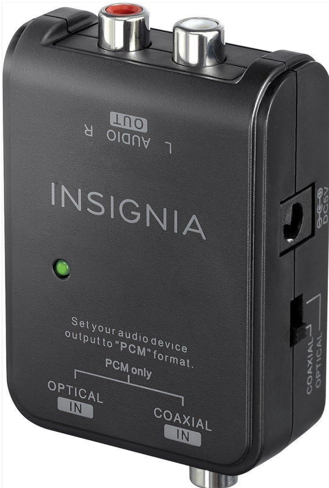
Image 3.2: Side View of the Converter. This image shows a side view of the Insignia NS-HZ313-C, detailing the DC 5V power input port and the "COAXIAL / OPTICAL" selector switch, which allows users to choose between the two digital input types.
