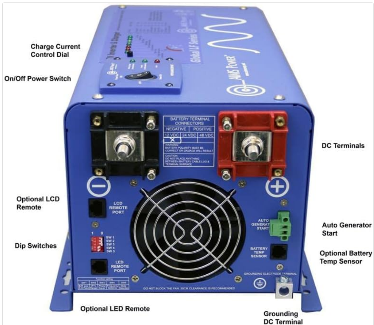
Figure 4.1: Rear Panel Connections and Controls
