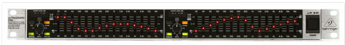
Image 1: Front panel of the Behringer Ultragraph Pro FBQ1502HD, showing the dual 15-band graphic equalizers, input/output level controls, FBQ feedback detection buttons, and power switch.
