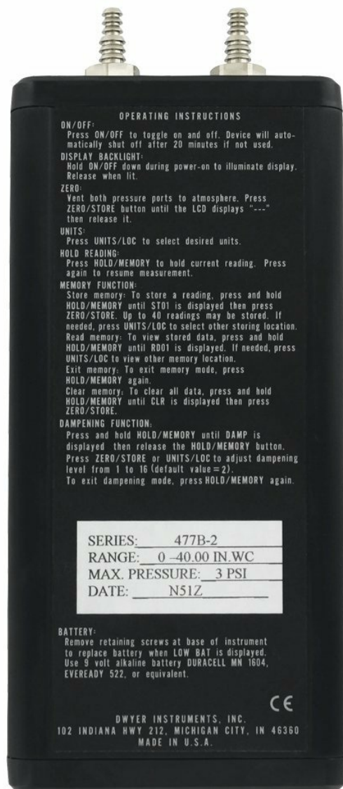
Figure 2: Back view of the Dwyer 477B-3 Digital Manometer, displaying key operating instructions and specifications.
