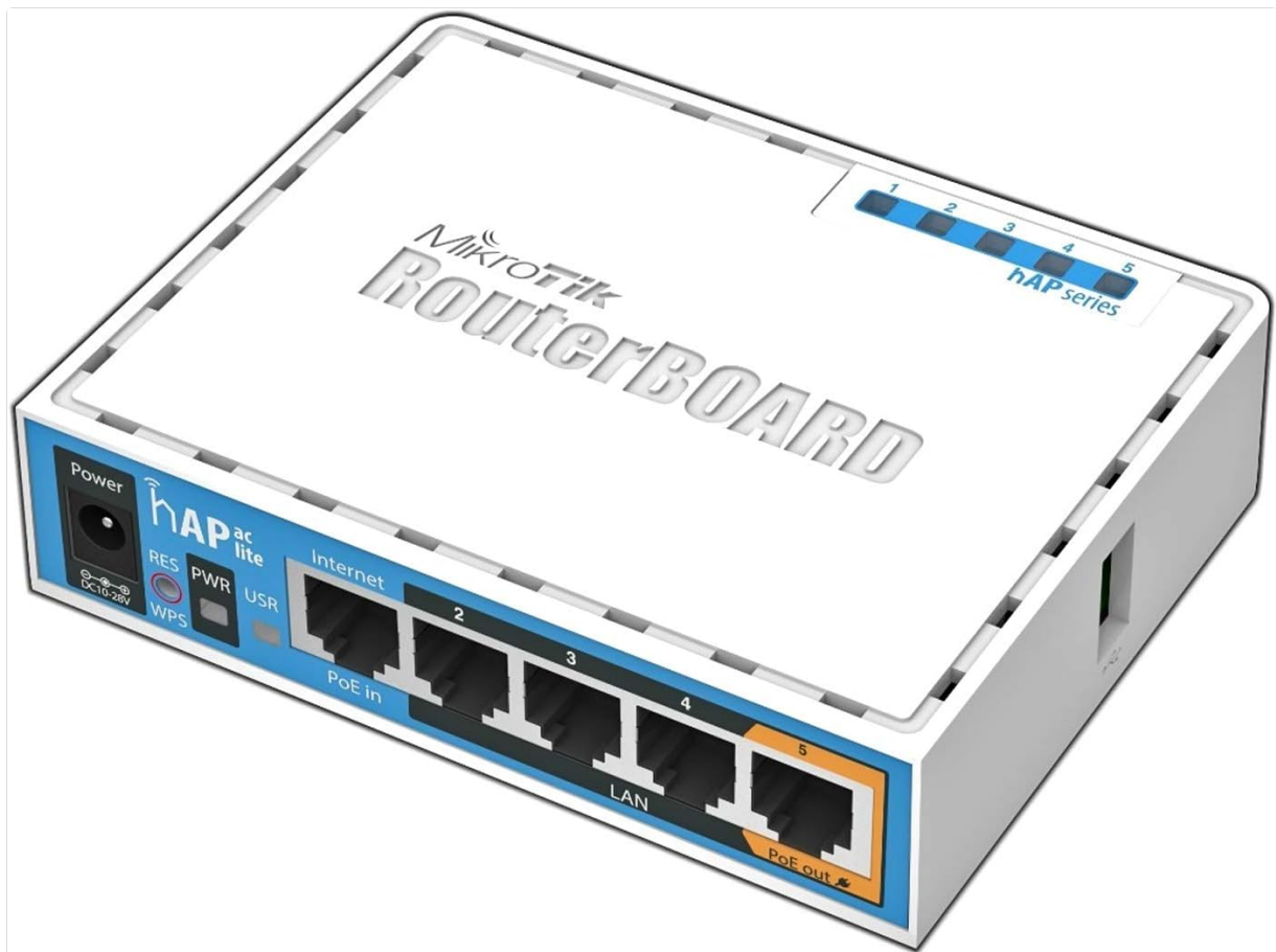
Figure 1: Front view of the MikroTik hAP ac lite with port and indicator labels.
