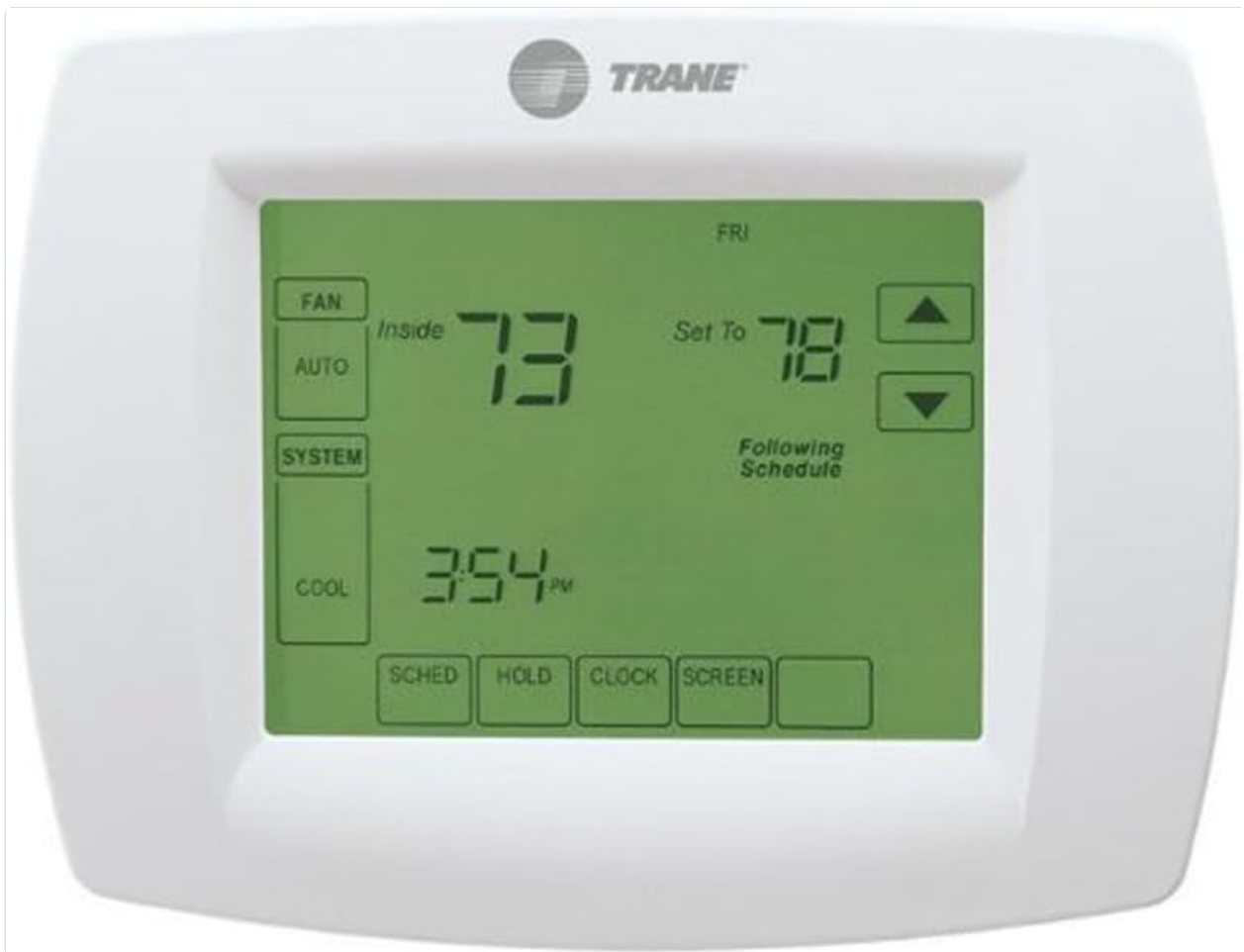
Image: Front view of the Trane Single-Stage Programmable Touchscreen Thermostat. It features a large, green back-lit digital display showing the inside temperature (73 degrees), the set temperature (78 degrees), the current time (3:54 PM), and various mode indicators like FAN, AUTO, SYSTEM, COOL, SCHED, HOLD, CLOCK, and SCREEN buttons.
