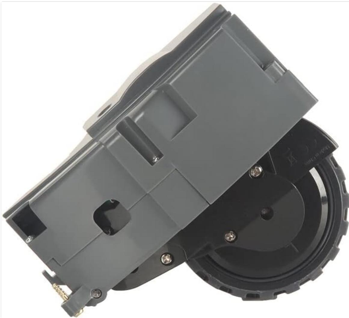
An image showing the iRobot Roomba Left Side Wheel Module, a grey plastic component with a black wheel attached, designed for robotic vacuum cleaners. This module is ready for installation or replacement.
