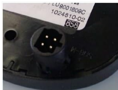
Figure 4.2: Close-up of the 4-pin electrical connector on the rear of the Webasto 1533 Digital Timer, highlighting the gold-plated pins for connection to the wiring harness.
