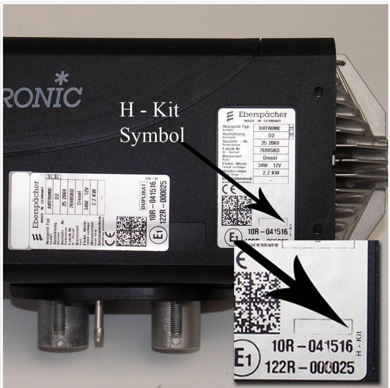
Figure 2: Detail of an Eberspächer Airtronic heater label, highlighting the "H-Kit" symbol which indicates compatibility with the High Altitude Kit.
