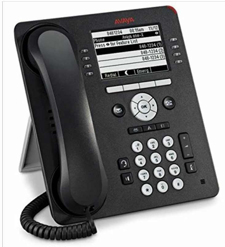
Figure 3.1: Front view of the Avaya 9608 IP Deskphone, highlighting the monochrome display and the four softkeys for interactive functions.
