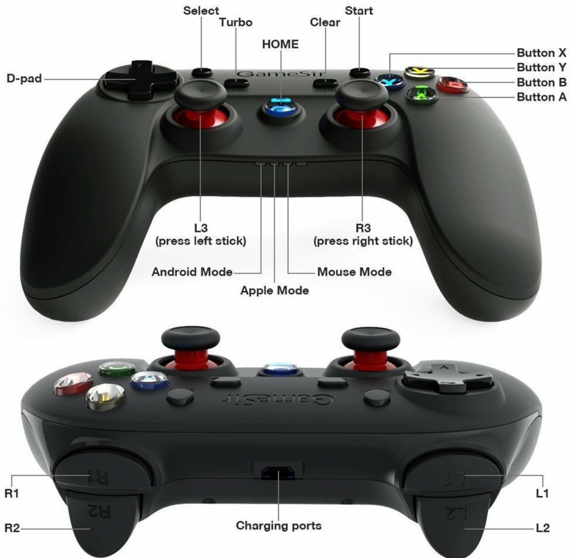
Image 3.1: Detailed diagram of the GameSir G3s Gamepad, highlighting all buttons and ports.
