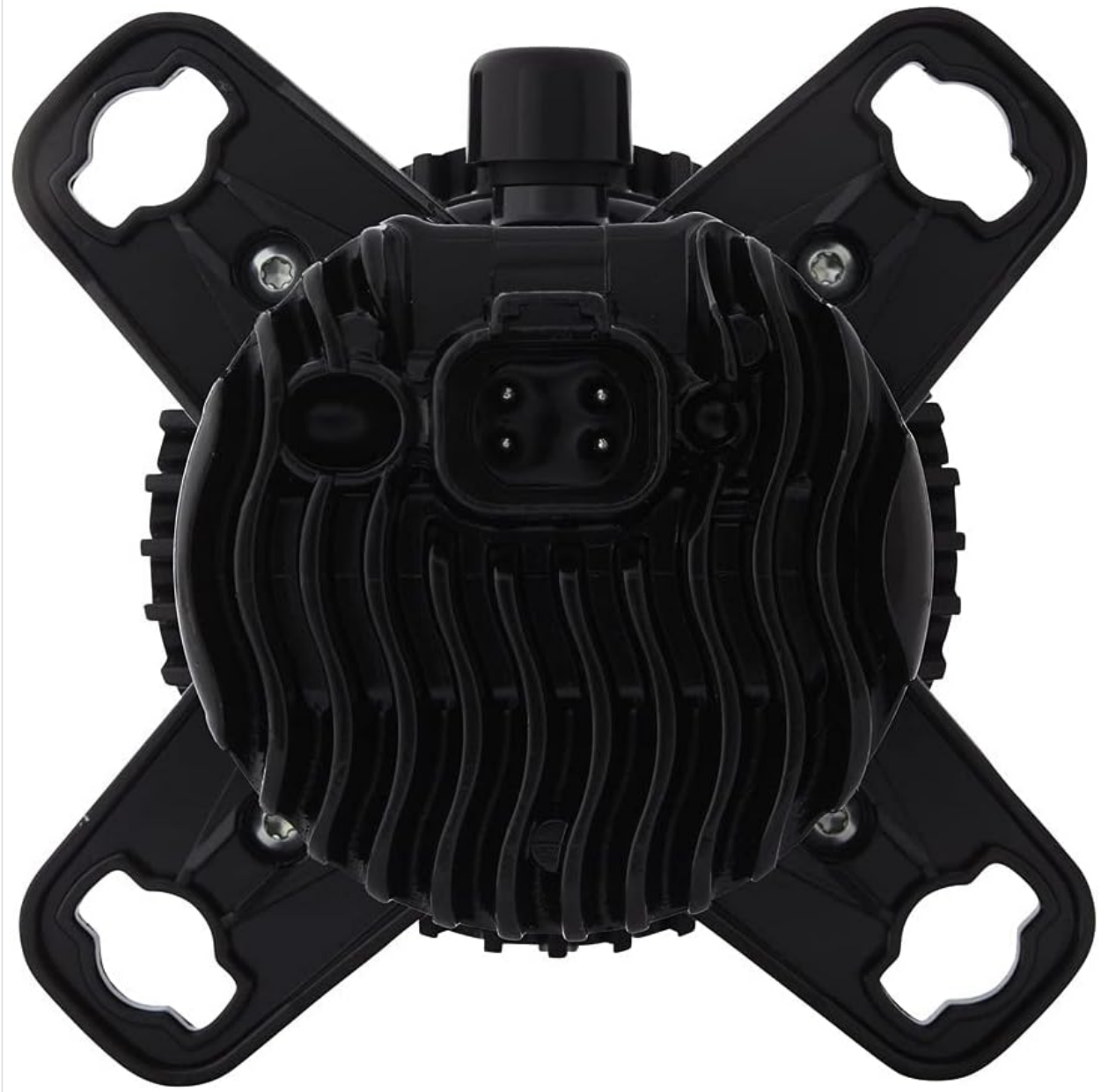
Image 4.3: Rear view of the headlight module, showing the DEUTSCH connector for electrical hookup.
