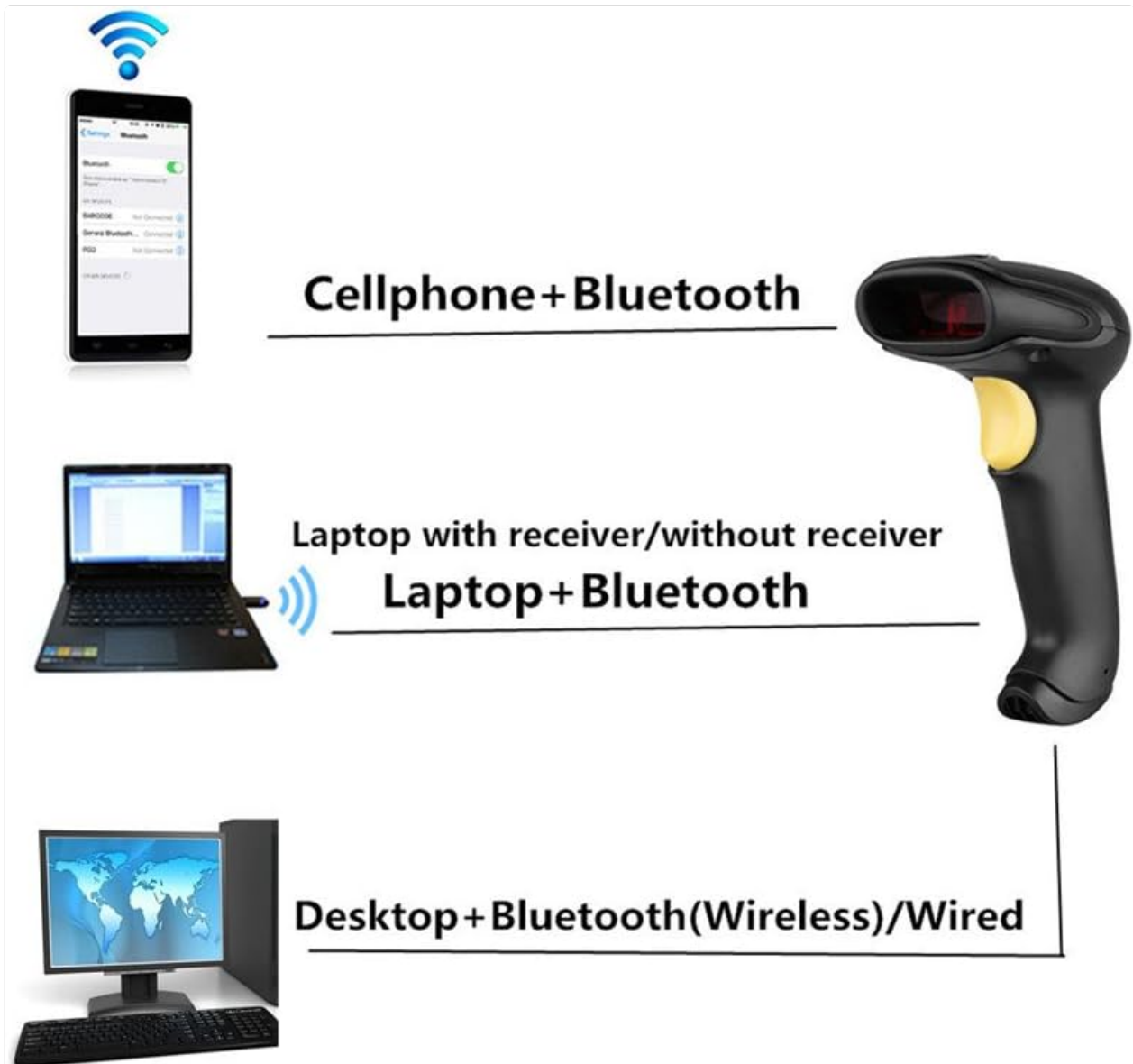
Figure 4: Diagram illustrating various connection methods for the barcode scanner, including mobile phone via Bluetooth, laptop with or without receiver via Bluetooth, and desktop computer via Bluetooth (wireless) or USB (wired).
