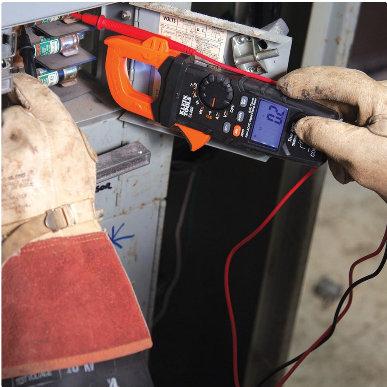
Figure 4: An electrician uses the Klein Tools CL800 to safely measure voltage across terminals in a circuit breaker panel, demonstrating practical application.
