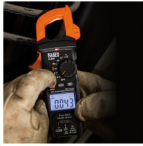
Figure 6: The Klein Tools CL800 is shown measuring temperature using its thermocouple probe, demonstrating its multi-functionality beyond electrical parameters.
