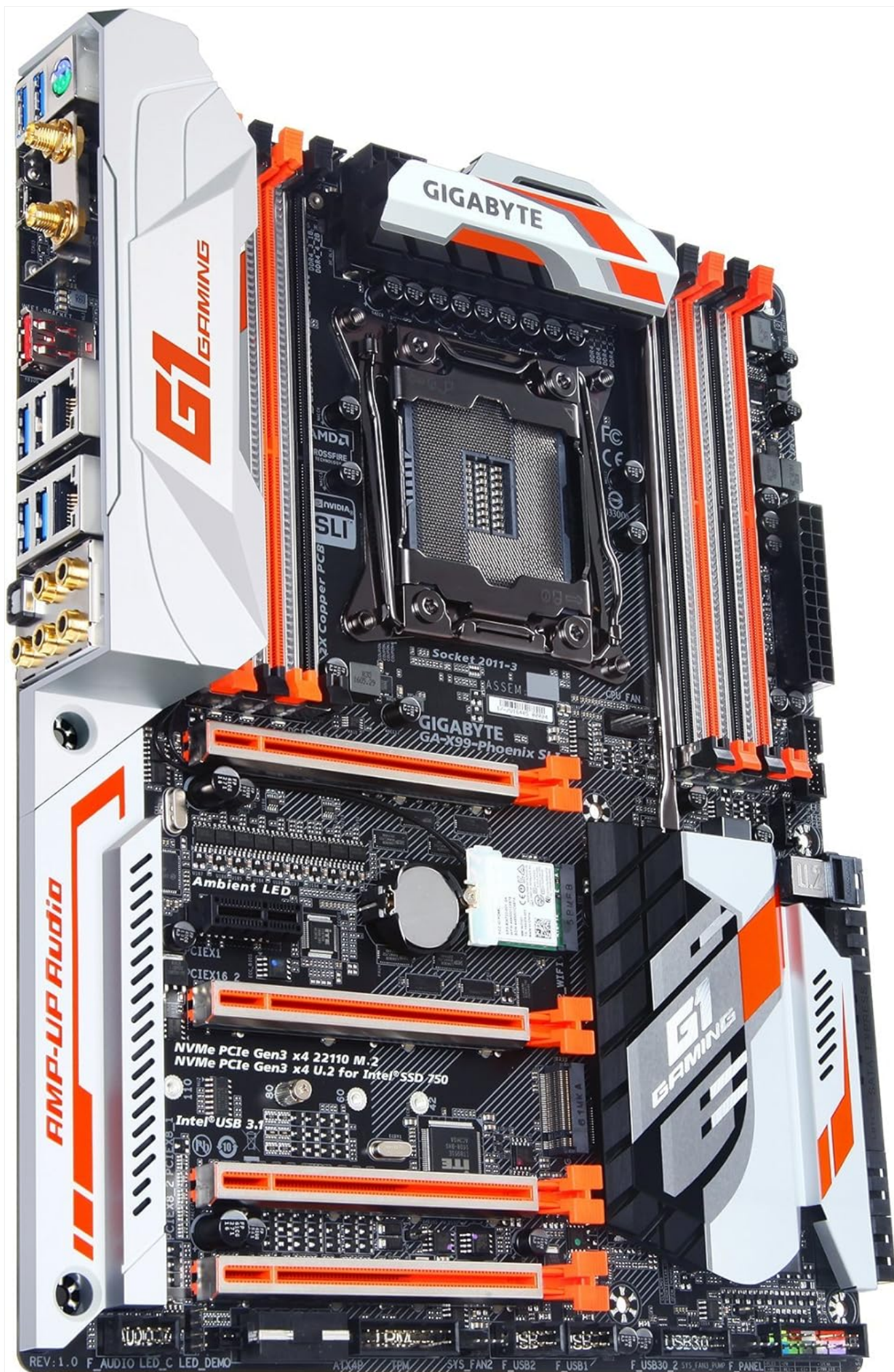
Figure 2: Angled view of the motherboard, highlighting the rear I/O panel and the layout of the PCIe and RAM slots.
