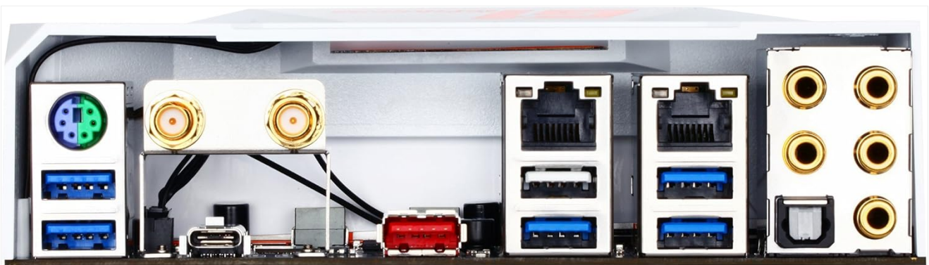
Figure 3: Close-up of the rear I/O panel, showing various ports including USB, Ethernet, audio jacks, and wireless antenna connectors.
