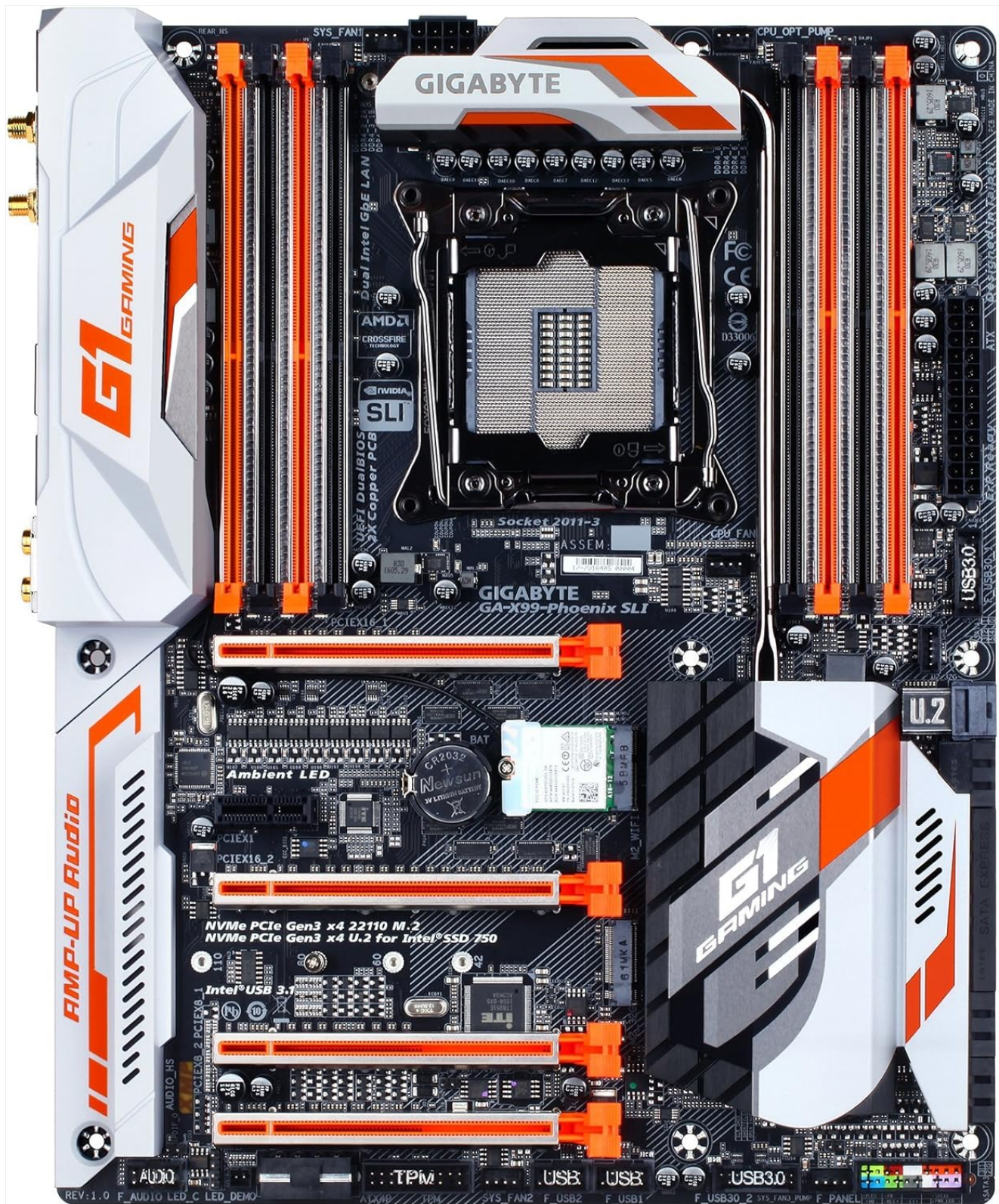
Figure 1: Top-down view of the GIGABYTE GA-X99-Phoenix SLI motherboard, showcasing its layout including the CPU socket, RAM slots, PCIe slots, and various connectors.
