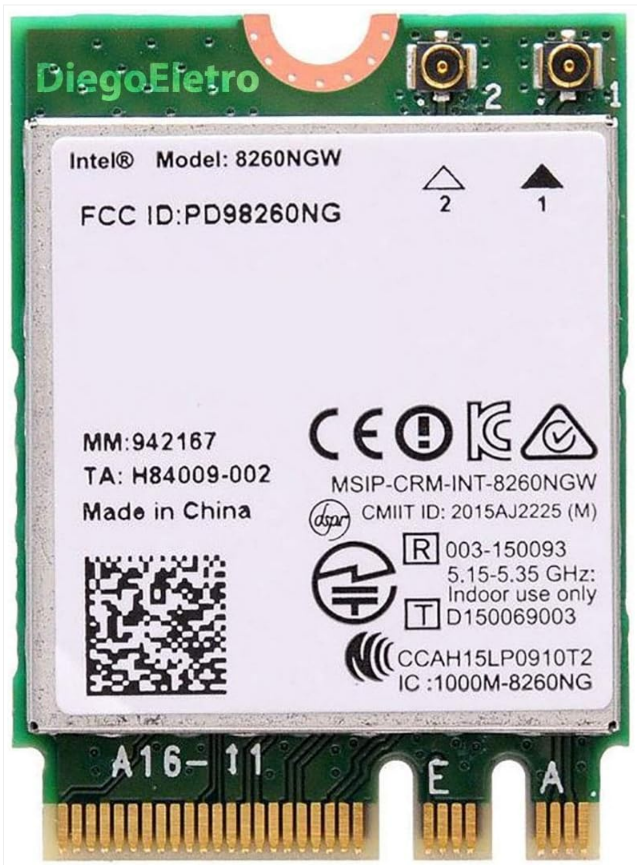
Figure 1: The Intel Dual Band Wireless-AC 8260 Wi-Fi Adapter. This image shows the compact M.2 form factor of the adapter, highlighting its various components and regulatory markings.
