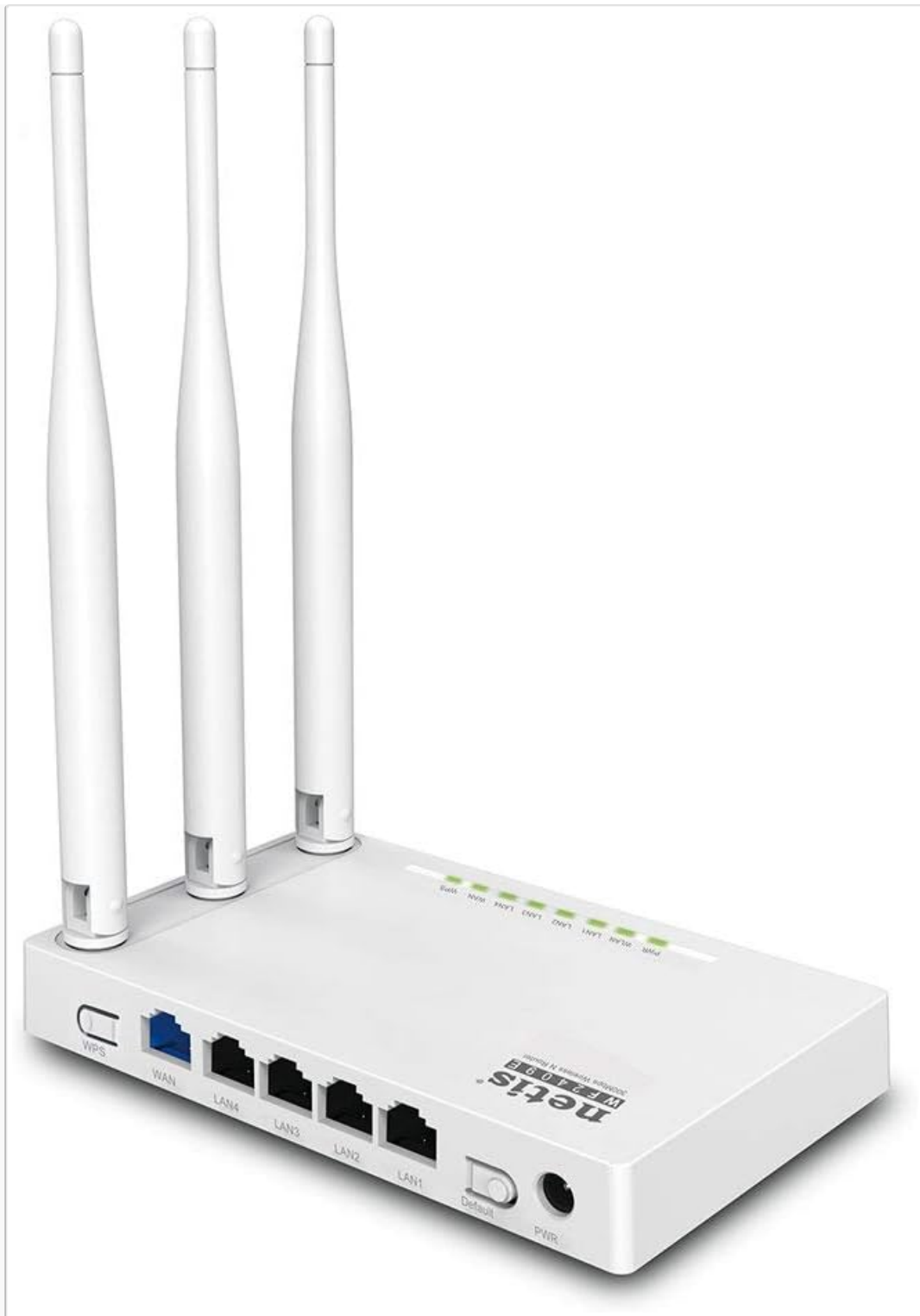
Figure 3.1: Netis WF2409E Router with its three antennas, front panel LEDs, and rear panel ports.
