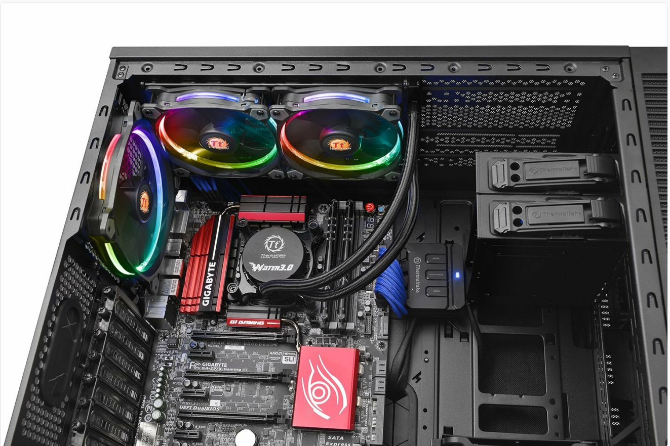
Figure 3.1: The Thermaltake AIO cooler fully installed within a desktop PC chassis, demonstrating proper placement of the radiator, fans, and pump unit.
