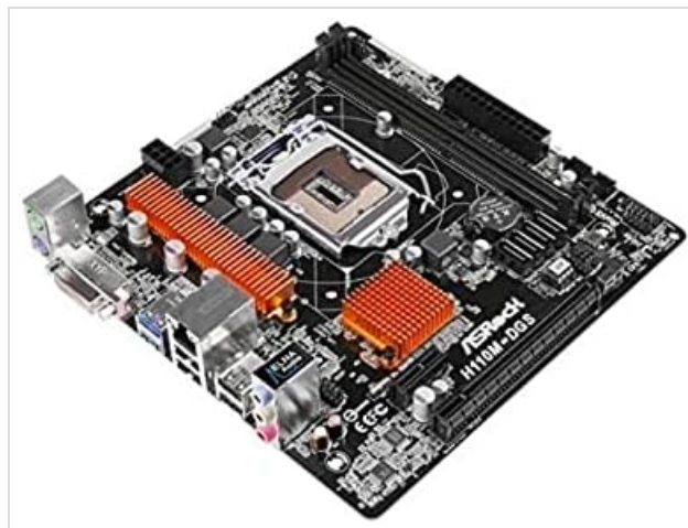
Figure 4.2: Angled view highlighting the CPU socket area, DDR4 memory slots, and the chipset heatsink.
