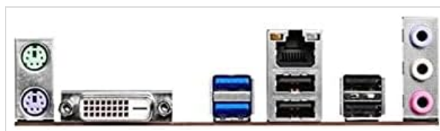
Figure 5.1: Rear I/O panel showing PS/2 ports, DVI-D, USB 3.0, USB 2.0, RJ45 LAN, and audio jacks.
