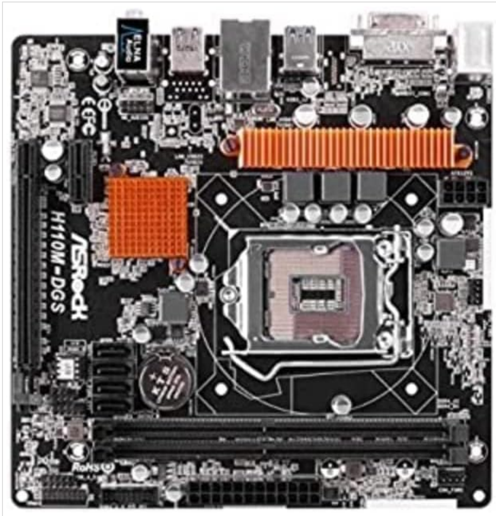
Figure 4.1: Top-down view of the ASRock H110M-DGS Micro ATX Motherboard, showing the CPU socket, RAM slots, PCIe slots, and various headers.
