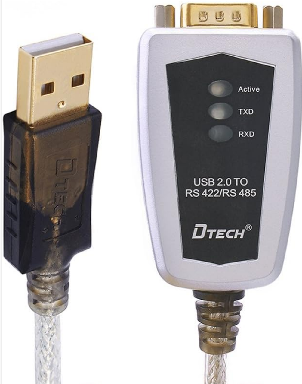
Image: The DTECH adapter highlighting the Active, TXD, and RXD LED indicators.
