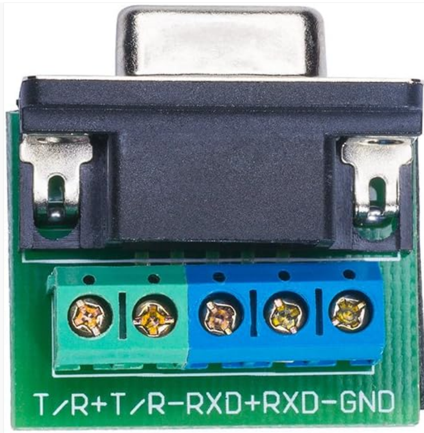
Image: Close-up view of the 5-position terminal board, showing screw terminals for T/R+, T/R-, RXD+, RXD-, and GND.
