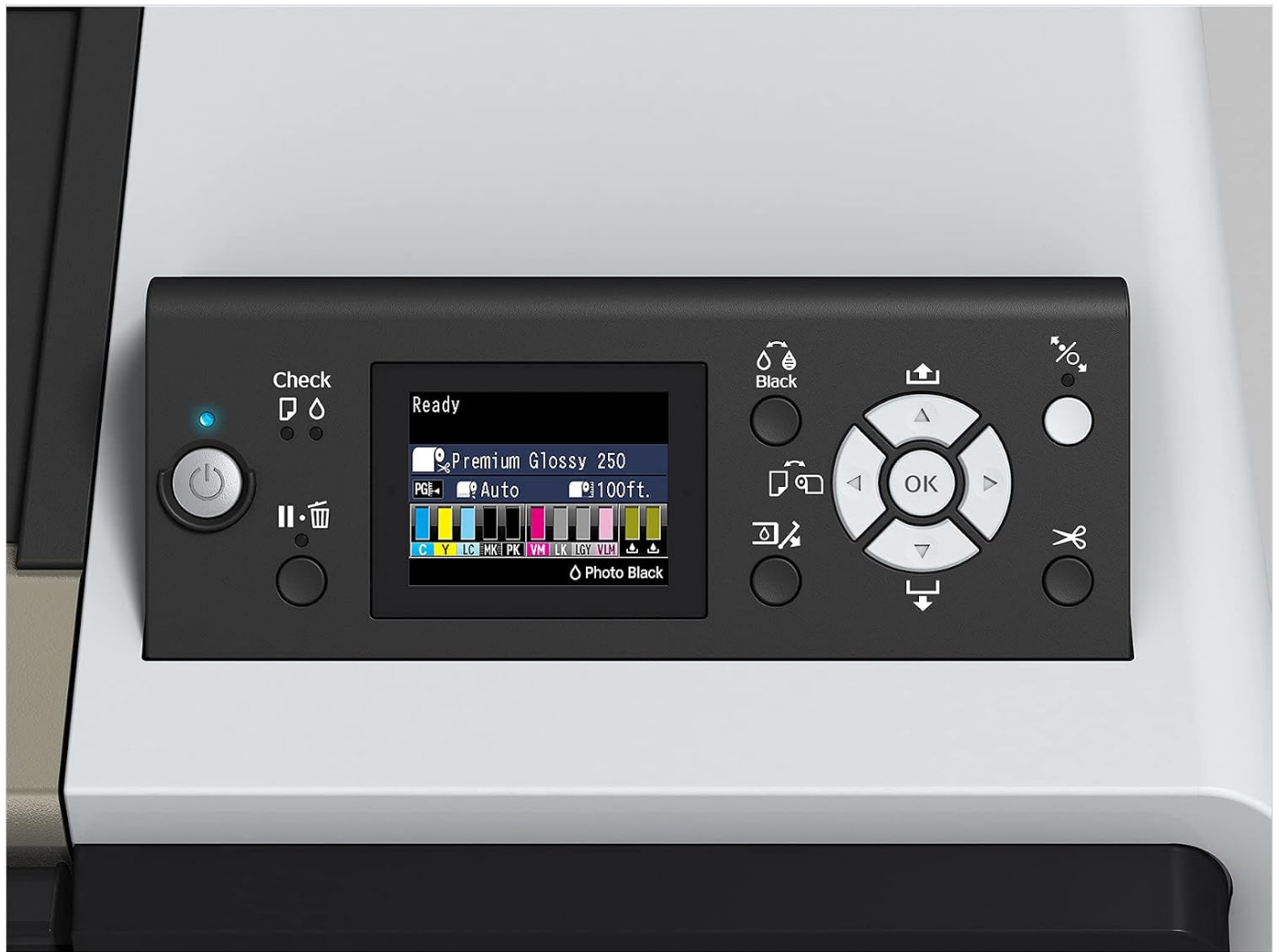
Image 4.1: Close-up of the Epson SureColor P8000 control panel. This image shows the LCD screen displaying ink levels and media type, along with navigation buttons and power button.
