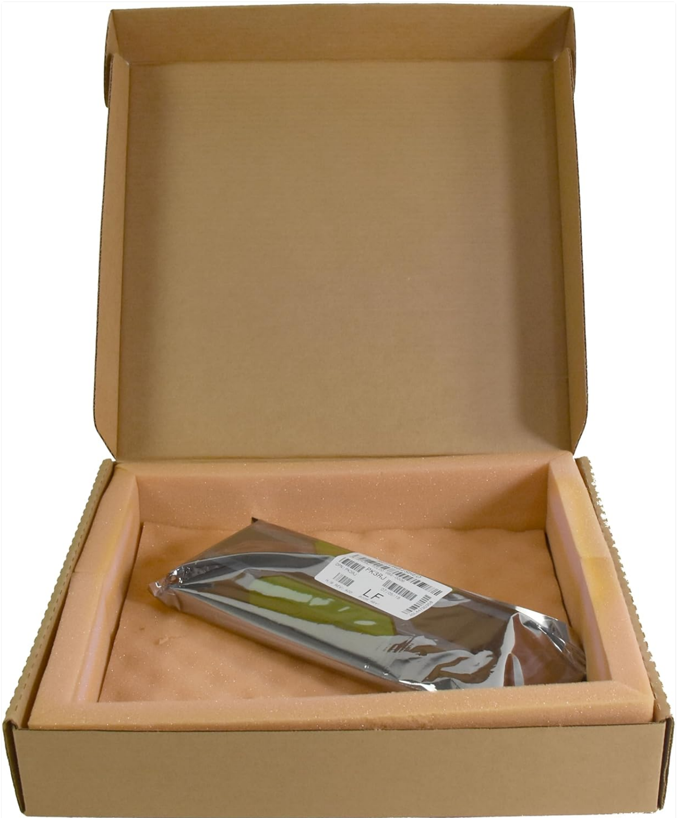
Figure 3.1: The HPE NVIDIA Tesla M60 GPU module as typically packaged in an anti-static bag within a protective box.
