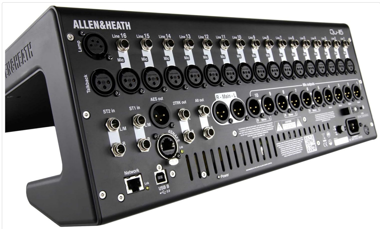
Figure 2: Rear panel of the QU-16C, highlighting the various input and output connections including XLR, TRS, USB, and Network ports.
