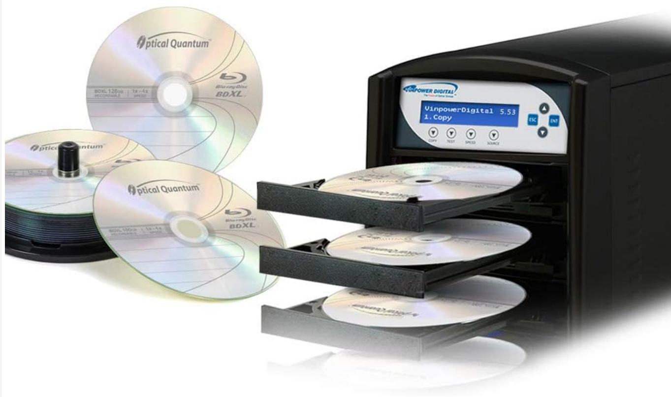
Image 4.3: The duplicator with its disc trays open, showing BDXL 100GB and 128GB discs being loaded or duplicated. A stack of BDXL discs is visible next to the unit.
