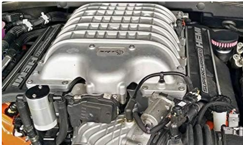
Image: Close-up view of the CFM Performance Baffled Billet Valve Cover Breather installed on a Hellcat engine's valve cover.
