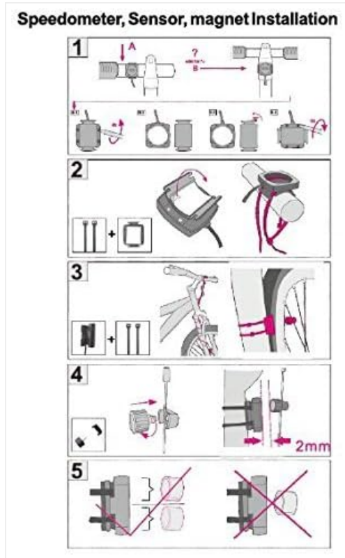
Figure 3: Comprehensive installation diagram illustrating the mounting of the computer, sensor, and magnet on a bicycle.
