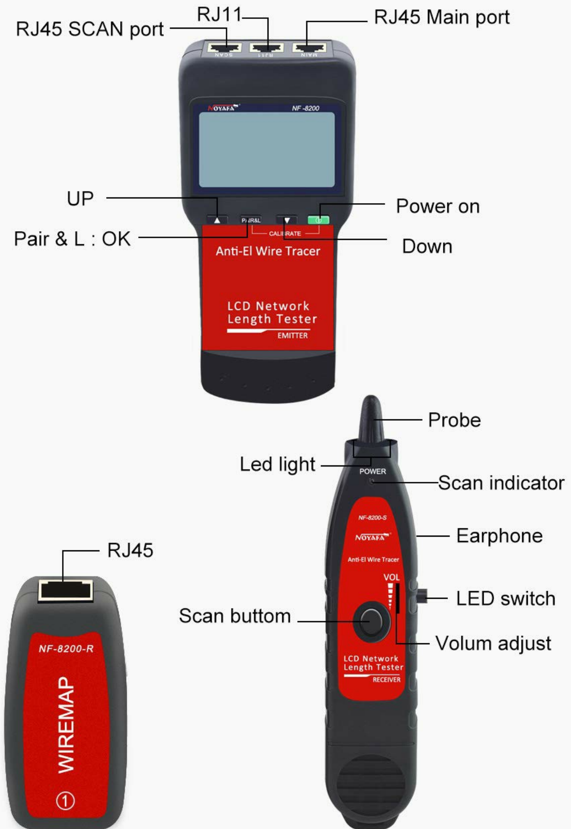
Figure 1: Overview of the NOYAF A NF-8200 Cable Tester components, including the main emitter unit, receiver probe, and remote unit.
