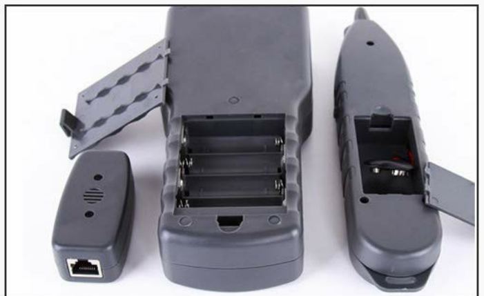
Power supply by 1.5v AAA battery
